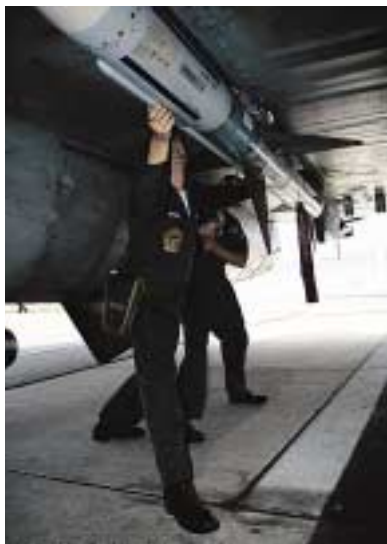
When attached to the launcher, two of the missile's 16-inch-wide triangular fins protrude into the bottom of the fuselage (photo by Ted Carlson).
